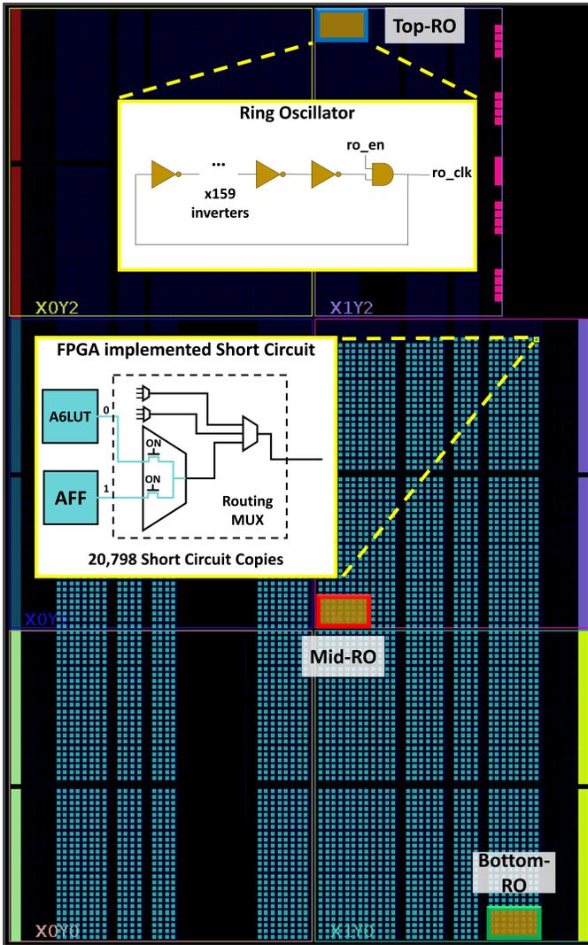
Figure 1: Three ring oscillators are used to measure slowdowns across the chip, during the “characterization” phase of the experiment. 20,798 shorts are used during the “burn” phase of the experiment, covering the lower two-thirds of the part. While both are shown in this figure, they are configured at different times.
