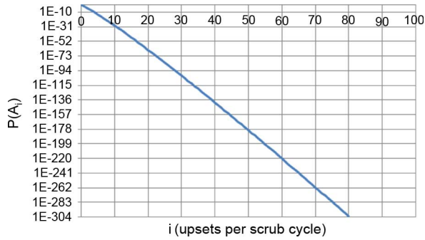
Fig. 2. Probability of i upsets per scrub cycle for a Xilinx Virtex-4 XQR4V5SX55 FPGA in solar max conditions in GEO with a 15 ms scrub period.
